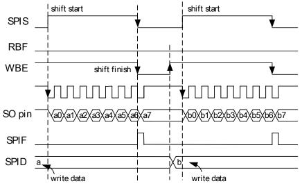
Fig. 15. Transmit Mode (8-bit, 1 word)
